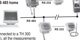
• When a Class 200 or 300 transmitters is connected to a TH 300 (with RS 232 connection), all the measurements can be given to the PLC/BMS via the RS 485, with only one address for the 2 transmitters.
